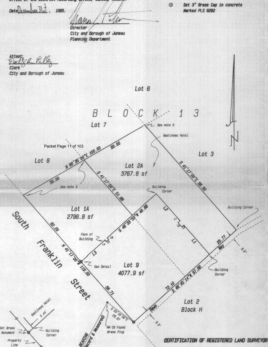
LINE DISTANCE BEARING 1 N 41 31 05 W 27.28 2 N 41'31'04"N 25.40 3 S 48 34 02 W 22.78 1.80 4 S 41"26"07"E 2.20 5 N 48 33 53 E 1.80 8 N 41 26 07 W 1.99 7 S 48 28 56 W 4.20 8 S 41°31'04"E 9 N 40 20 56 E 1.99
