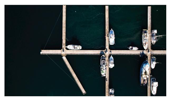
Docks and Harbors (D&H) staff responded to the site and assisted patrons on the night of the storm to relocate their vessels to adjacent stalls. At daylight, staff returned with a larger crew and removed the remaining vessels away from the damaged fingers and installed temporary cables to restrain the fingers and prevent further damage.
